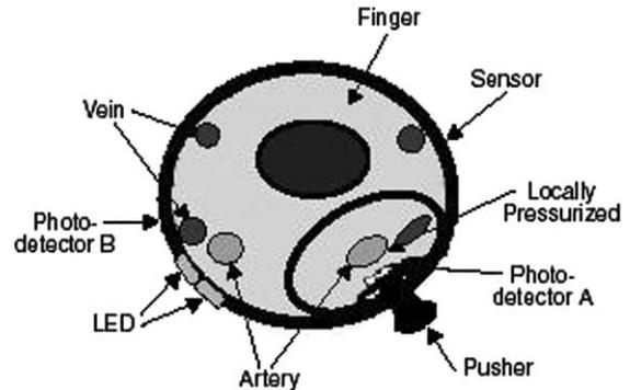
Fig. 5. The schematic of a locally pressurized sensor band.
