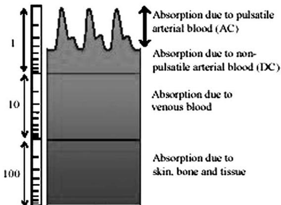
Fig. 2. Illustrative representation of the relative photon absorbance for various sections of the finger. The dc component is significantly larger than the ac component.
