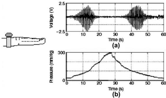
Fig. 4. (a) PPG signal amplitude and (b) pressure at the photodetector.
