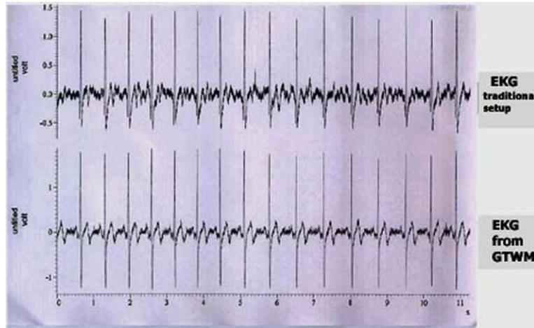
Fig. 9. EKG waveforms from traditional setup (above) and GTWM (bottom).
