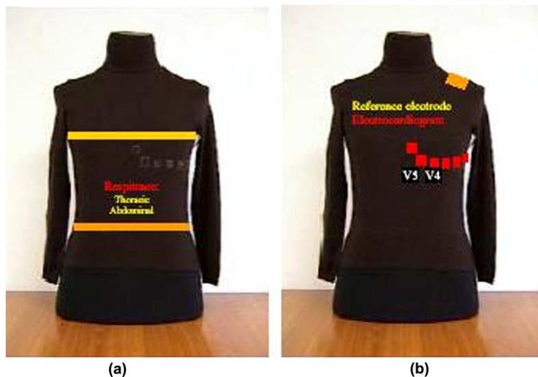
Fig. 11. Positioning of fabric sensors on a smart shirt for RT (a) and ECG (b).
