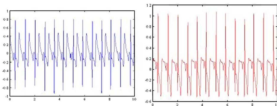
Fig. 12. (a) ECG detected with bi-layer fabric and (b) ECG detected with standard electrode.
