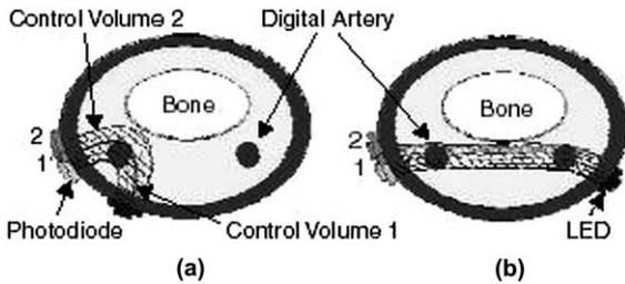
Fig. 3. (a) For the reflective illumination method, movement of the photodiode relative to the LED (position 1 to position 2) leads to a photon path that no longer contains the digital artery. (b) For the transmittal illumination method, movement of the photodetector relative to the LED still contains photon paths that pass through the digital artery.
