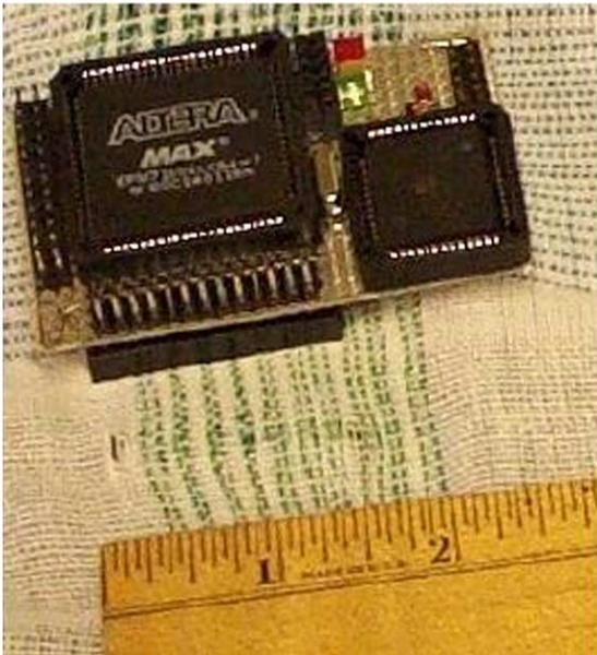
Fig. 10. Prototype board,  $2.8'' \times 1.8''$ , containing the FPGA and microcontroller.
