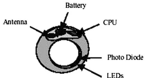
Fig. 1. Conceptual diagram of the ring sensor.
